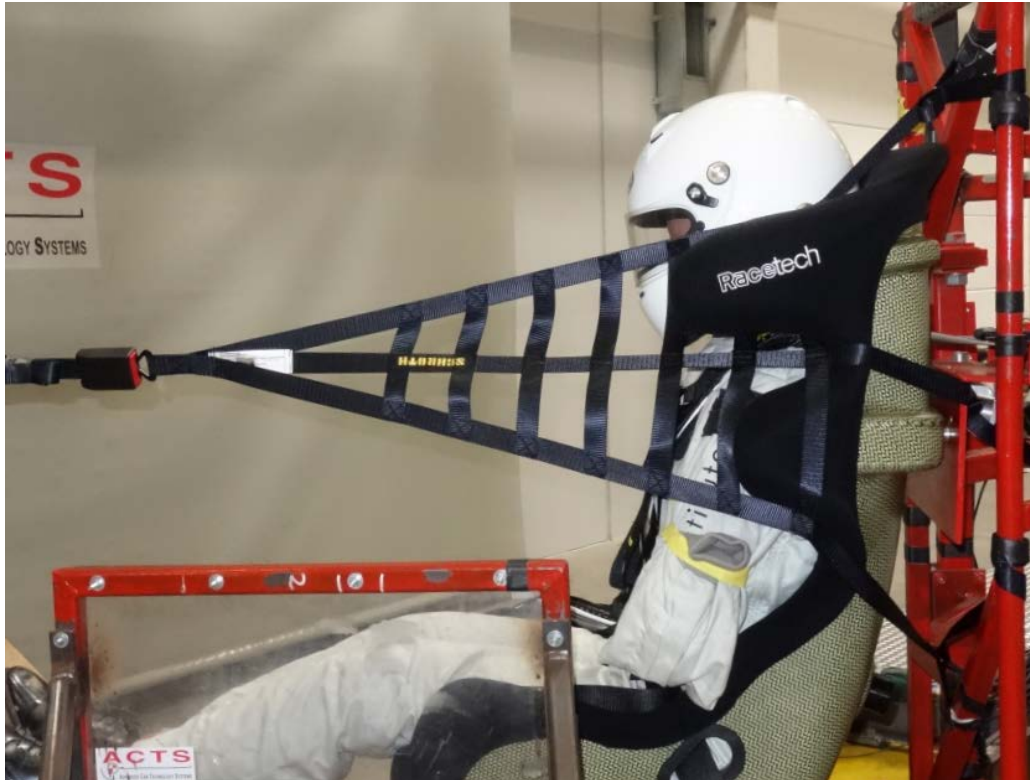
Figure 3: Photograph showing upper-strap inside the seat-side-head (external view)
