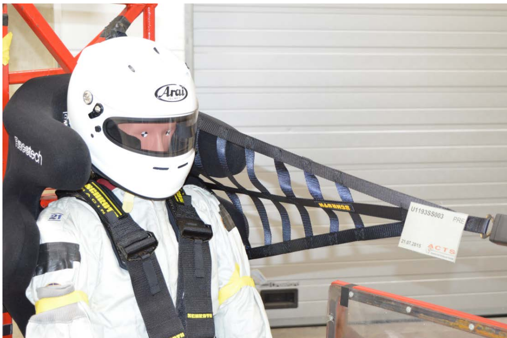
Figure 4: Photograph showing upper-strap inside the seat-side-head (internal view)
