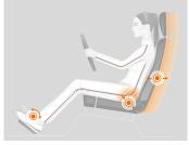
**5.** Adjust the extendable seat cushion so that the thighs rest on it to just above the knee. Rule of thumb: two to three fingers Space between the edge of the seat and the hollow of the knee.
