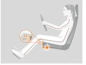
2. Rest your shoulders as closely as possible on the backrest. Set the backrest tilt so that the steering wheel is easy to reach with slightly bent elbows. Shoulder contact must be maintained when the steering
