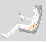
**3.** Set the seat height as high as possible. This ensures an unobstructed view to all sides and all displays on the instrument panel.
